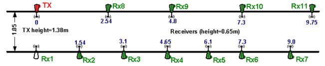
Fig. 3. Locations of transmitter & receivers
