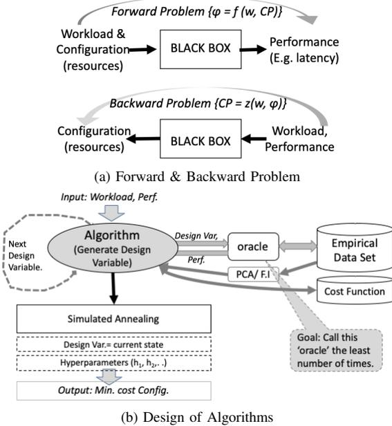
Fig. 2: Basic Approach: Design of Solution.
