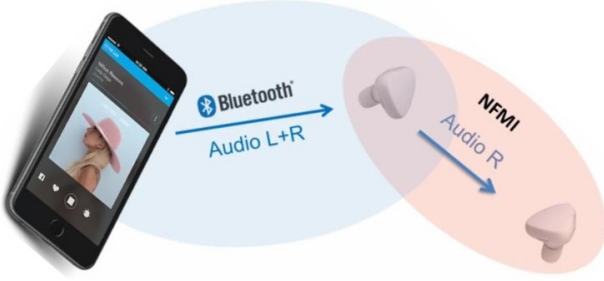
Fig. 13. Combined BLE and NFMI based communication [146].
