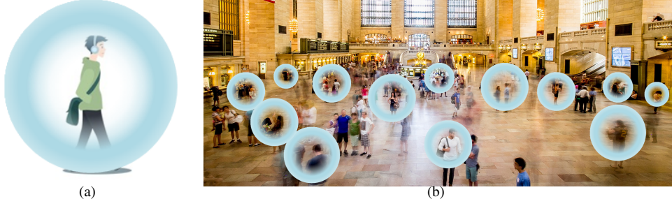
Fig. 1. (a) A magnetic bubble around an user's PAN. (b) This small bubbles ensure a significant amount of spatial reuse of the same frequency in a crowded area.
